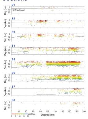
Most aftershocks are confined between the ground surface and the MHT shear zone, and the bottom of the aftershock is consistent with the 3D MHT model.
