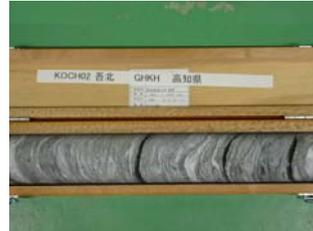
core on the bottom of Hi-net borehole
